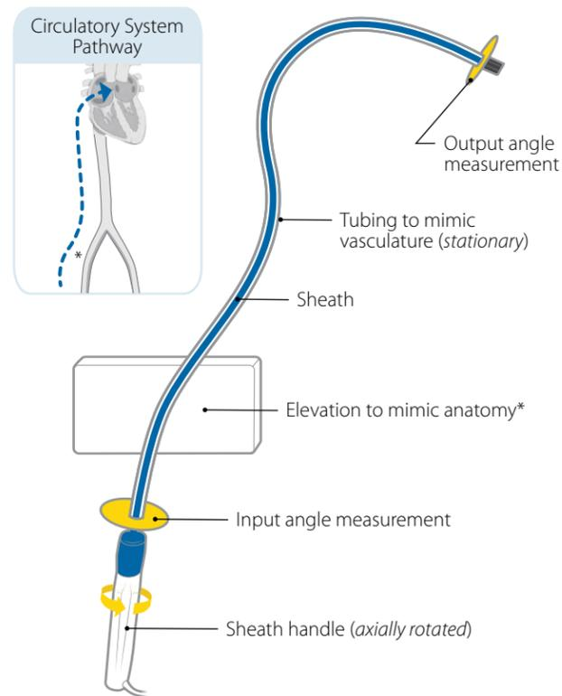
Figure 1 Axial rotation test set-up
