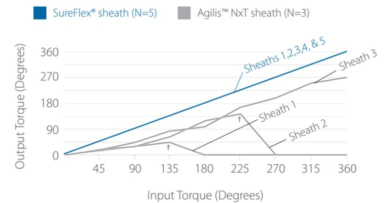
Figure 3 Individual sheath torque transfer (axial rotation) performance (\*indicates sheath breakage)
