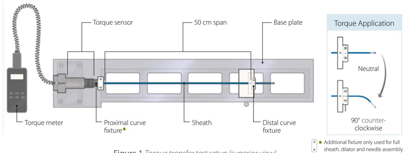
Figure 1 Torque transfer test setup (superior view)
