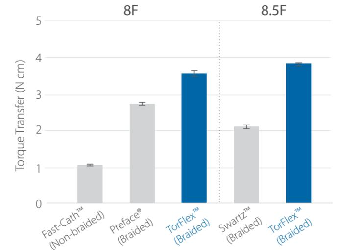
Figure 3 Torque transfer of sheath and dilator set
