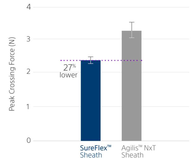
Figure 3. Peak crossing force comparison (mean ± standard error for 10 SureFlex™ sheaths and 8 Agilis™ NxT sheaths,  $p < 0.001$ )
