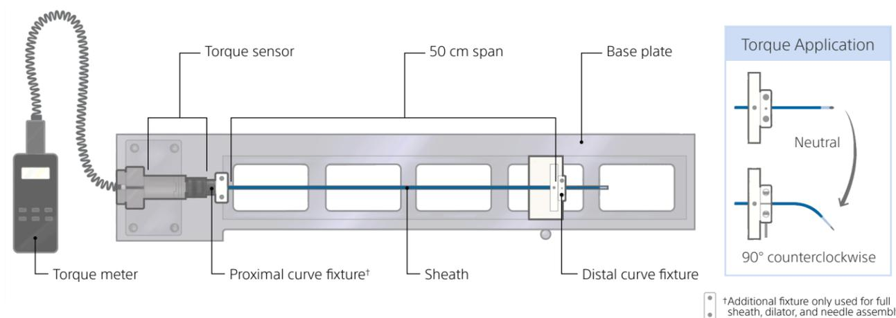
Figure 1. Torque transfer test setup (superior view)
