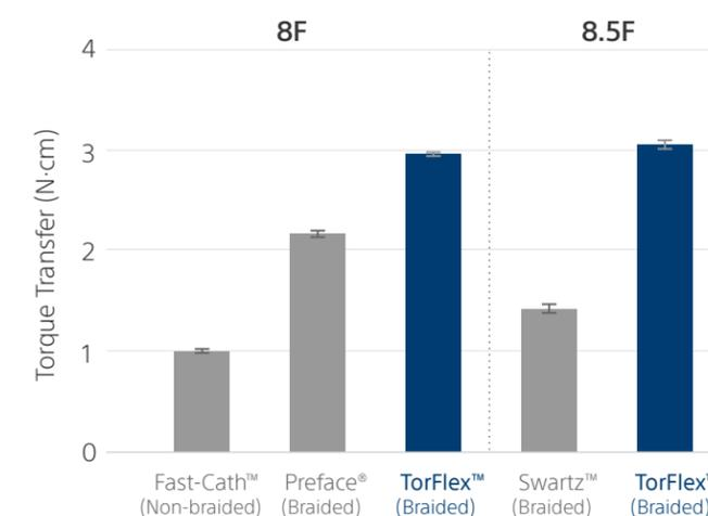
Figure 2. Torque transfer of sheaths
